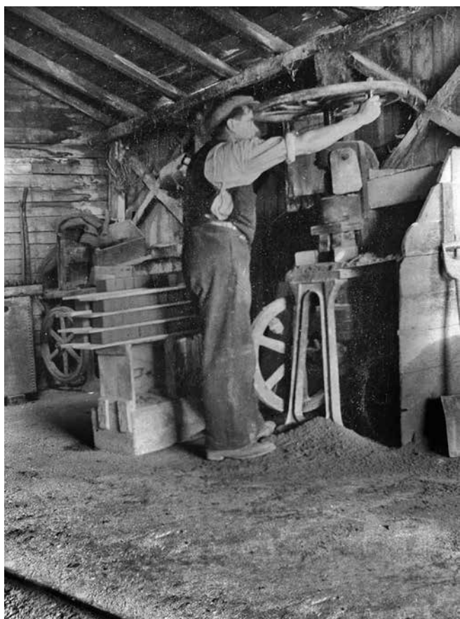
Hearthstone processing factory at Colley Hill c1910. This was the only Surrey hearthstone mine where processing was done at the mine. Ground hearthstone, possibly mixed with a small quantity of 'binder', is being compressed in a mould into rectangular blocks for sale. The factory was destroyed by a fire shortly before the mine closed
